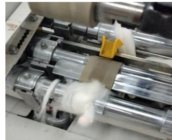
Figure 15: Random Lapping on the Bottom Rolls
