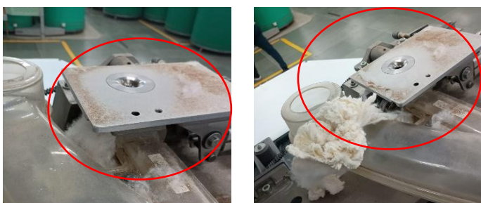
Figure 11: Fiber Choking at the Coiler Calendar Roll with Kitti Accumulation
