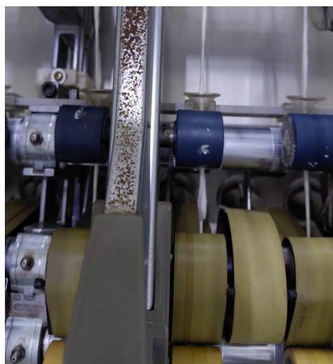
Figure 33: Sticky Deposition on Back Top Rolls
