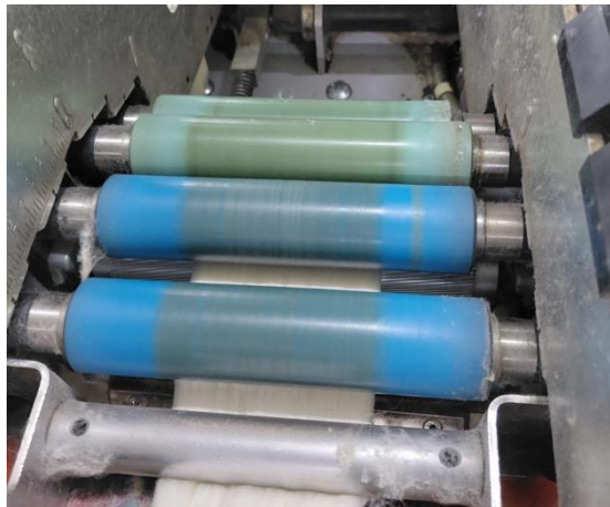
Figure 32: Change in Drafting Roller Coating Condition
