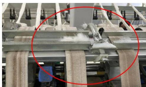
Figure 31: Fly Accumulation on Top Clearer
