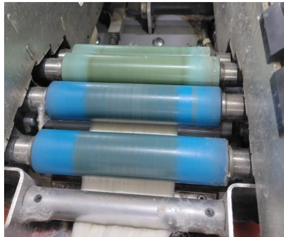
Figure 1: Change in Drafting Roller Coating Condition
