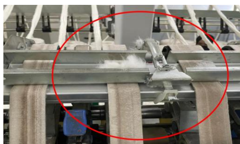
Figure 3: Fly Accumulation on Top Clearer
