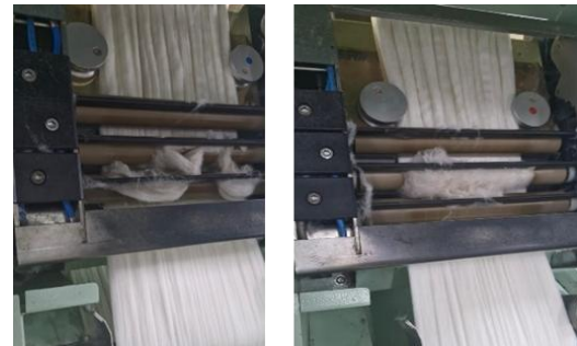
Figure 4: Higher Fly Accumulation in Omega Lap Draw Box
