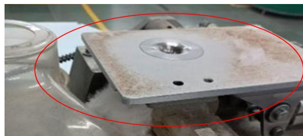
Figure 2: Fiber Choking at Coiler Calendar Roll
